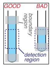
• Solid particles in a liquid sample present huge areas of solid/liquid interface that disrupt B<sub>0</sub> homogeneity. To get good data quality, particles must be removed, usually by filtering.
