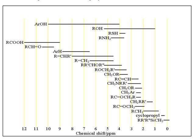
• It is sometimes handy to know how to approximately convert ppm to Hz. For <sup>1</sup>H nuclei on a 400 MHz instrument, the conversion is 400 Hz/ppm. On a 500, it's 500 Hz/ppm. For <sup>13</sup>C on a 400 MHz instrument, for which <sup>13</sup>C's are resonating at 100 MHz, it's 100 Hz/ppm. You get the idea.
