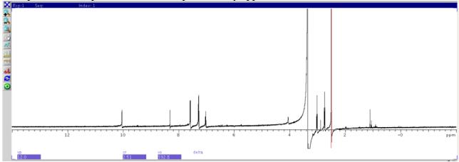
• The peaks in this spectrum are "properly phased"; you can draw an imaginary line through the baseline on one side of the peak and it will meet up with the baseline on the other side of the peak:
