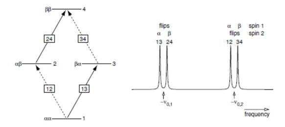
On the left, the energy levels of a two-spin system; the arrows show the allowed transitions: solid lines for transitions in which spin 1 flips and dotted for those in which spin 2 flips. On the right, the corresponding spectrum; it is assumed that the Larmor frequency of spin 2 is greater in magnitude than that of spin 1 and that the coupling  $J_{12}$  is positive.
