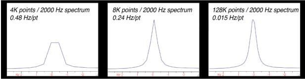
• One caveat to zero-filling: If an FID is too short, it will give rise to "wiggles" at the base of the peaks, the sharpest peaks being most affected. Zero-filling does not fix this problem, and it is usually best to fix the "wiggle" problem by increasing the acquisition time.
