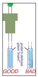
• The centers of the inner and outer surfaces of the tube may not coincide well. Poor positioning of the sample in the coil and nonuniformity of the glass wall thickness create shimming problems. "Concentricity" is the measure of the difference between the two circles' centers. Tubes with higher "MHz" ratings have better concentricity.
