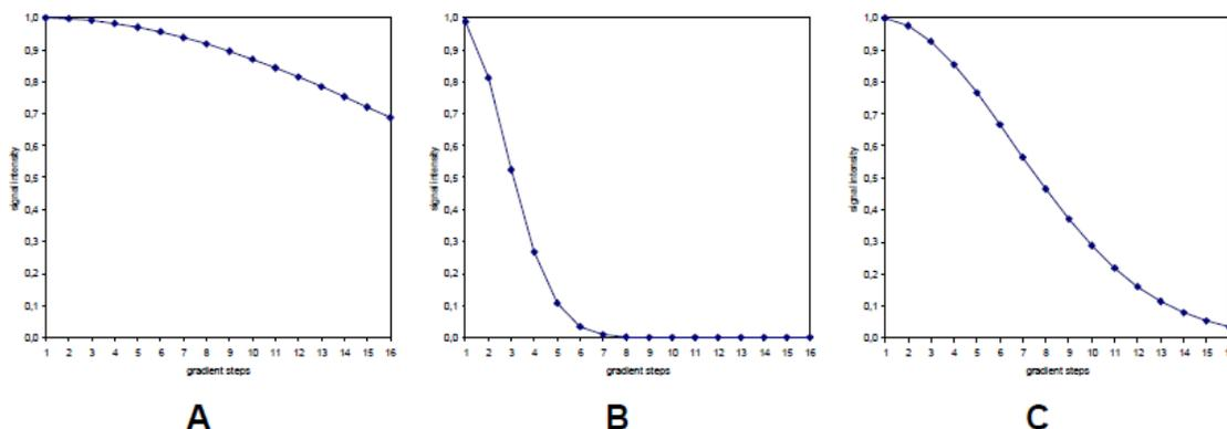
**Figure:** Simulated diffusion decay curves by varying the gradient strength  $g$  from 2 to 95% in 16 steps for the same diffusion constant, but with different selection for  $\Delta$  and  $\delta$ . They are chosen too small (A), too big (B), and properly (C) to sample data points along the whole decay curve.
