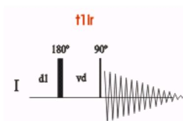
The basic pulse sequence consists of an 180° pulse that inverts the magnetization to the -z axis. During the following delay, relaxation along the longitudinal plane takes place. Magnetization comes back to the original equilibrium z-magnetization. A 90° pulse creates transverse magnetization. The experiment is repeated for a series of delay values taken from a variable delay list. A 1D spectrum is obtained for each value of  $vd$  and stored in a pseudo 2D
