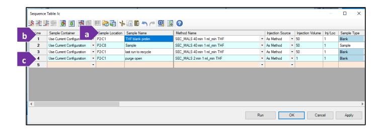
6. Click on (a) 'Apply' to apply sequence changes. And then (b) 'Run' at the bottom of the sequence table.
