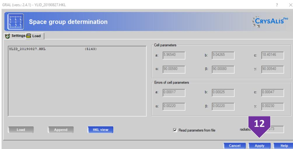
13. Investigate the centering absences. Recall that the first row corresponds to the total number of reflections you would expect to collect for the condition listed in the column. The second row indicates how many of the symmetry equivalent reflections that you collected violate that condition. This cell appears to be primitive. Click “Apply”.
