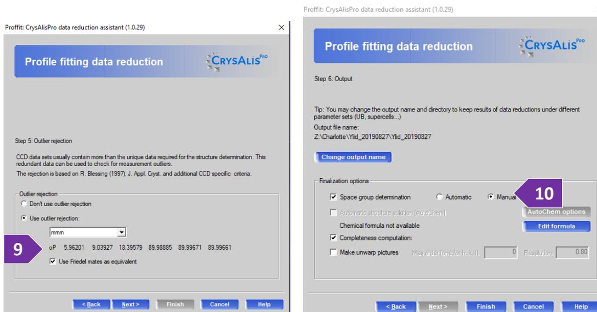
11. Click “Finish”, Watch the integration and monitor the output in the tab. The software runs through the dataset twice. First, the software locates the peaks (marked “+”) and develops a 3D peak profile. Second, the UB matrix and 3D profile are used to calculate the position and intensity of each reflection (3D integration & fitting). The peaks are marked by “integration masks” that give a visual idea of the size and possible overlap of the peaks.
