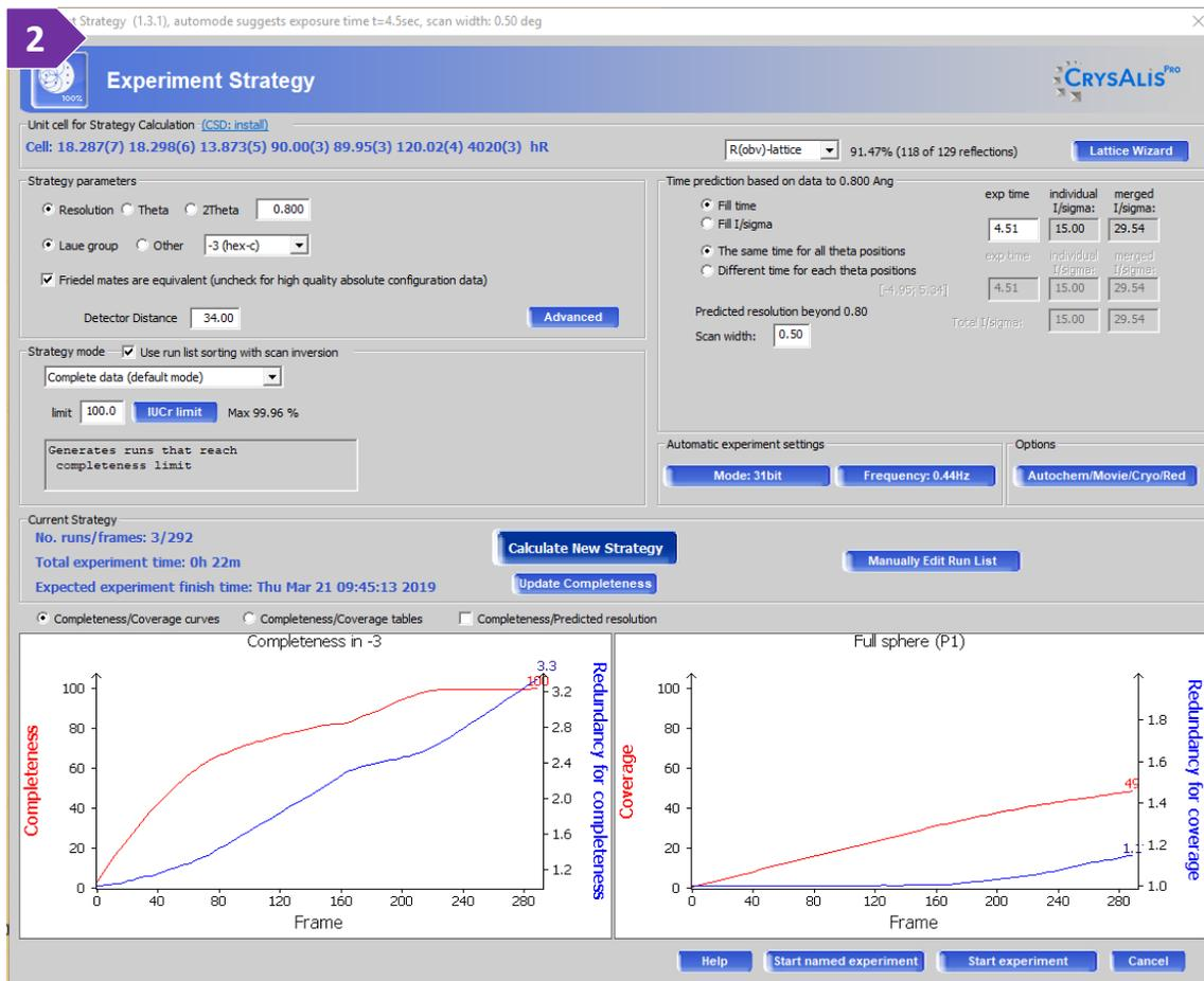
1. Cell constants will appear at the top left corner of the strategy window. If there are any hits in the CSD that match these cell constants, you will be able to see these reported structured by pressing on the corresponding link. Select the lattice type that you want to collect under
