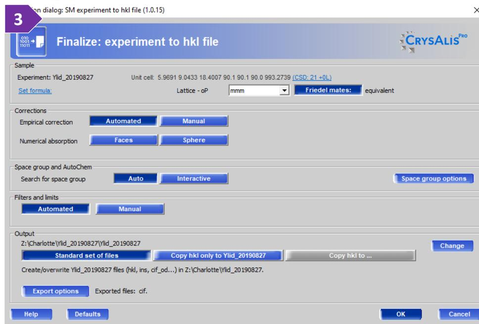
4. Under the “Corrections” section, verify that “Empirical correction” is set to “Automated”. This will apply the Blessing method of absorption correction to the reflections. You may also include faces. Click “OK”.
