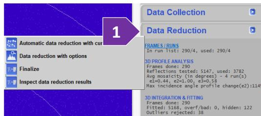
2. Ensure that don't use filter is checked if lattice is not known. If the lattice is centered (A, B, C, I, F, R), click *use filter for:* and select the correct centering. Make sure Normal data reduction is checked and then click “Next”.
