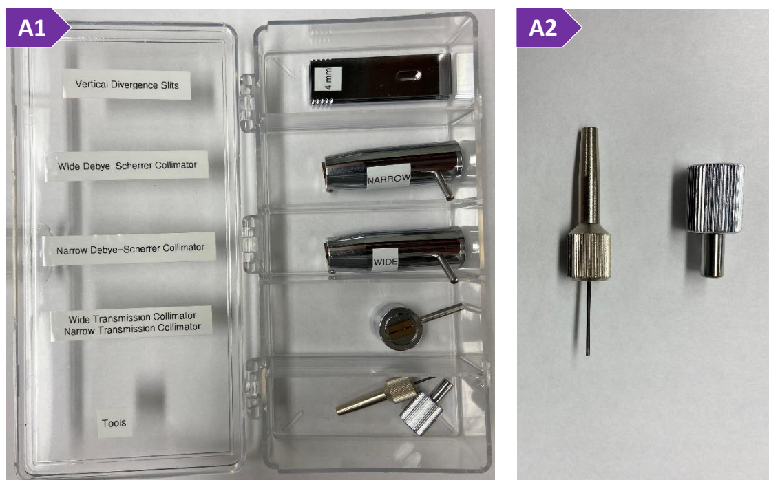
Figure A1. Toolbox containing the various accessories needed for the alignment of the goniometer head. Figure A2. Wrenches that can be used for adjusting the alignment screws on the goniometer head
